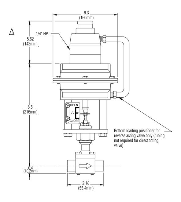
Additional height by 708SHTP only (Top mounted positioner only available on 14M actuators)
